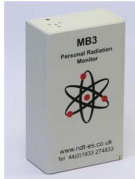
The MB3 provides audible and visual warning of the presence of ionising radiation. The audible alarm is a high pitched beep tone and the repetition rate of the tone will increase in proportion to the dose rate. At a dose rate of 7.5 $\mu$ Sv/hr and above the beep tone changes to a shrill chirp and again the repetition rate of the chirp will increase in frequency if the dose rate increases.
